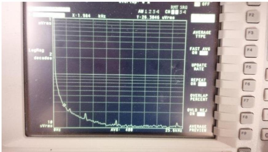
**Figure 8: Noise [ $V/rtHz$ ] vs Frequency [Hz] plot from signal analyzer**
